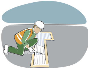
5) Positioning and adjustment of ground surface indicator tiles
