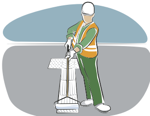
6) Pressing indicator tiles on the ground surface
